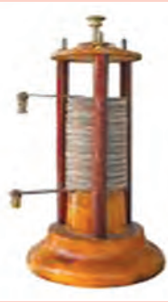
Volta's simple electric cell
