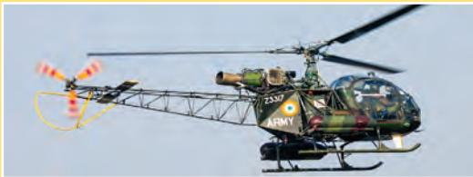
**Cheetah :** Single engine turboshaft, FAC / casevac helicopter of French origin.
