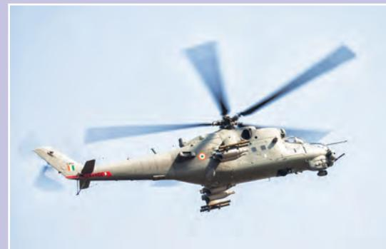
**MI 25/MI 35 :** Twin engine turboshaft, assault and anti armour helicopter.
