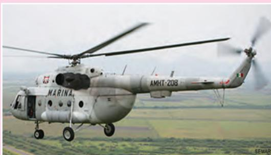
**MI 17 V-5 :** They are equipped with state-of-art navigational equipment, avionics, weather radar and are NVG-compatible.
