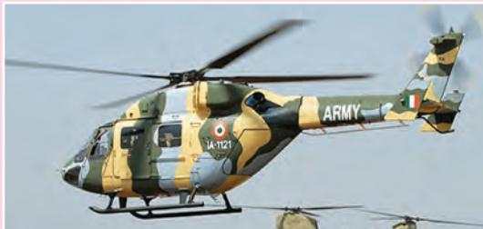
**Dhruv:** This is an Indian origin helicopter for transportation. This helicopter can work in mountainous area effectively up to the height of 6000 m.
