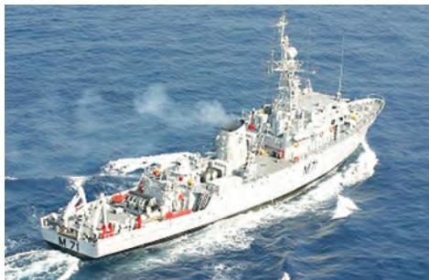
**Mine Countermeasure Vessel:** Also known as a minesweeper is a small naval warship designed to counter the threat posed by naval mines. Minesweepers keep waterways clear for shipping.
