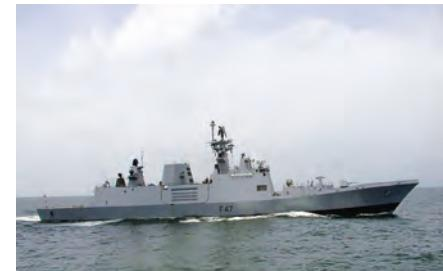
**Corvette:** It is a fast, lightly armed warship which is smaller than a frigate and larger than a coastal patrol craft often armed for antisubmarine operation.
